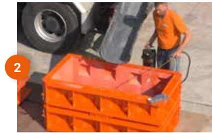
2 Applying oil into the mould
